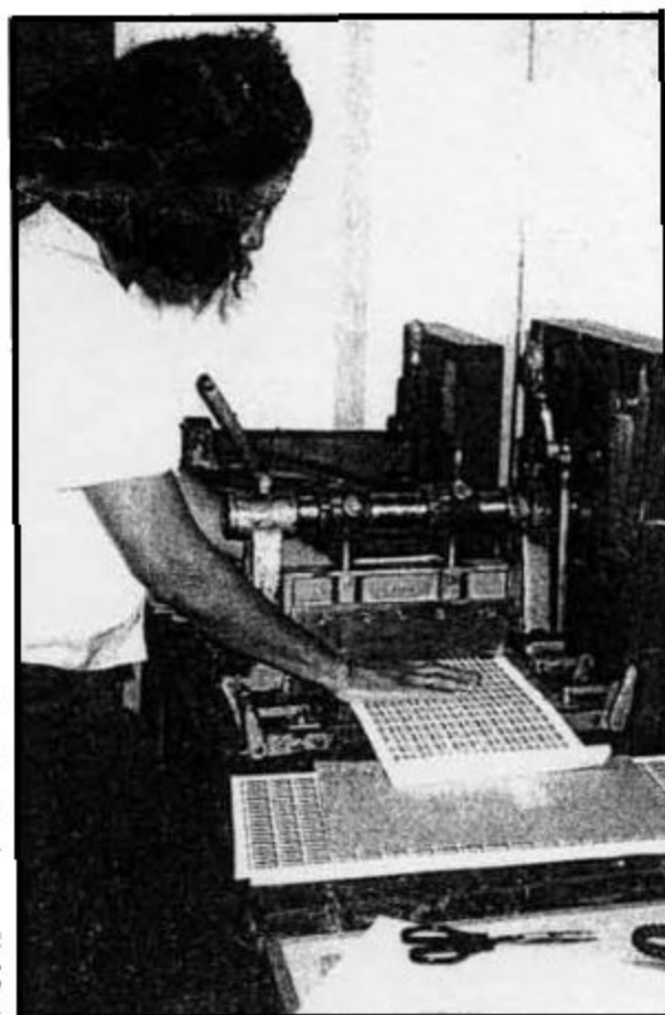
Perforating perfin on 24p and 18p stamps at Reading using Sloper's original machines.
