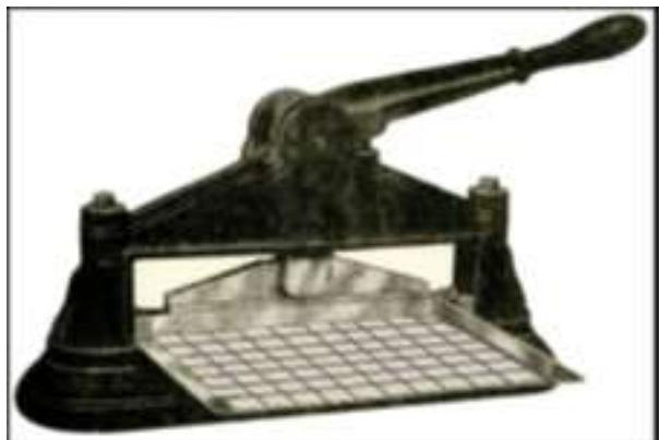
**Fig. 2: Cummins perforator with 10 dies on the head.
